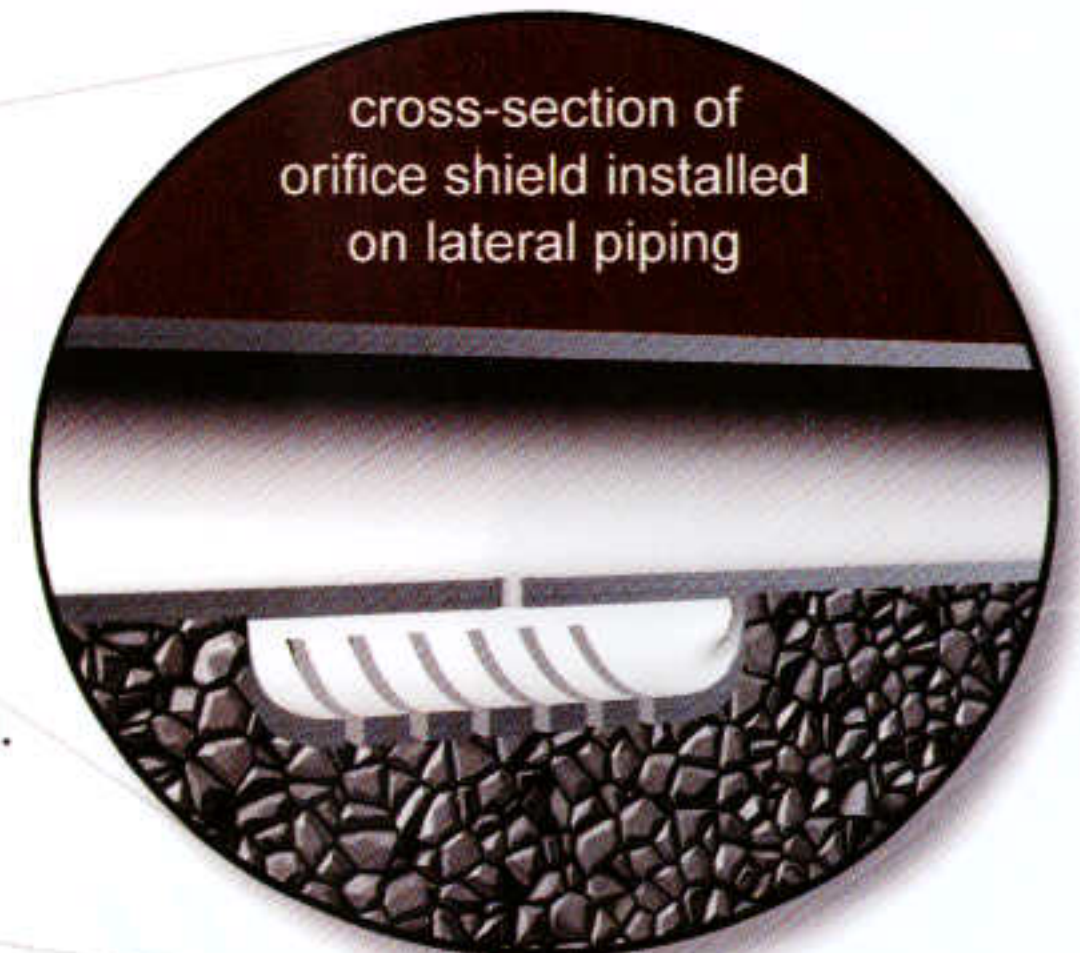
illustration of orifice shield installed over lateral piping
